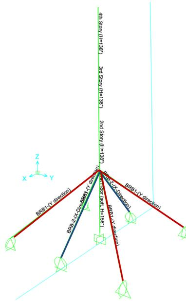
Figure 4. Simplified stick model of the structure for use in non-linear time-history analysis.
