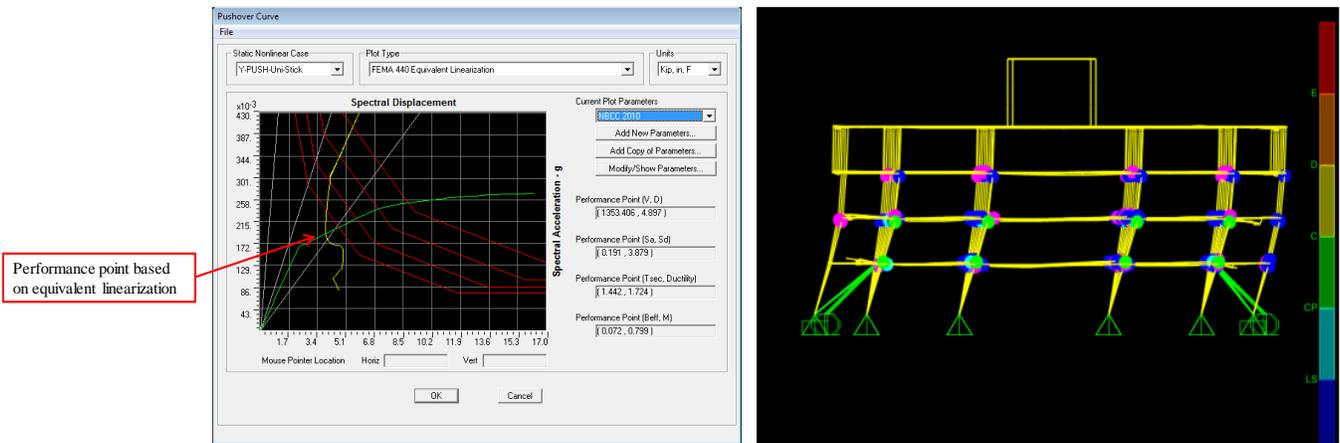
Figure 7. Equivalent linearization method in SAP2000 and hinge formation throughout the structure at the performance point.
