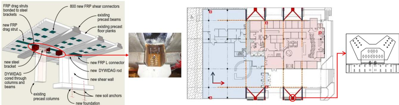
Figure 9. FRP drag strut to steel bracket connection to provide continuity of load path through columns and into the shear walls (left side of figure); layout of drag struts (red dotted lines) relative to BRBs and slotted connection at base of V-configured BRBs.
