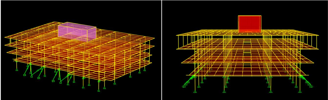
Figure 2. Views of the 3-dimensional model created in SAP2000, four storey steel moment frame portion of building.
