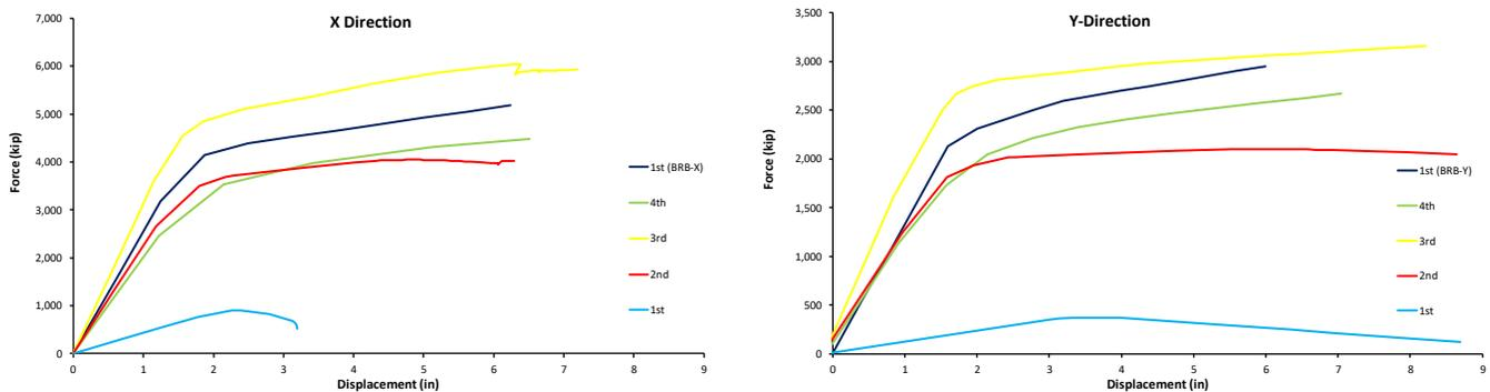
Figure 3. Non-linear storey backbone curves obtained from non-linear pushover analysis on each level, each orthogonal direction, including new BRBs on 1<sup>st</sup> level.
