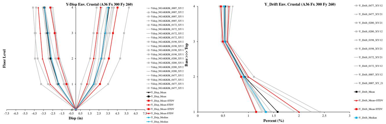
Figure 5. Displacement (left side of figure) and drift (right side of figure) profiles obtained from 2-dimensional time-history analysis for the suite of crustal ground motions.
